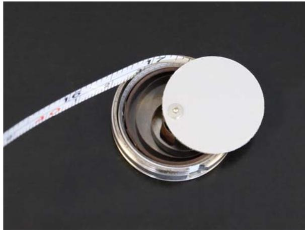
7. At this point you can safely remove the screw and guard disc.
