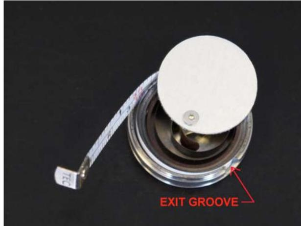
6. The measuring tape is actually two pieces, the measurement strip and the spring steel winding. They are attached together by means of a tab and slot. Note the orientation of this connection point as you are unwinding the tape. Continue to rotate both the tape and the winding out of the housing until it is completely unwound.
