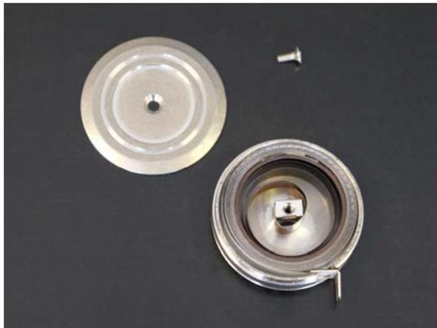
3. Remove the replacement tape and the guard disc from the packaging. There is a thin clear protective film on both sides of the guard disc, remove it and discard.
