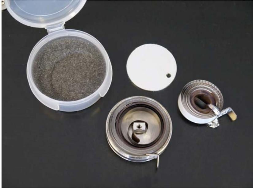
4. You must first remove the existing measuring tape from the housing. The safest method is to use the included guard disc that comes with the replacement tape, as its purpose is to keep the measuring tape inside the housing during the removal process. Attach the disc using the original cover screw and fasten it to the center hub. You do not need to tighten the screw, as the disc needs to rotate freely during the removal process.
