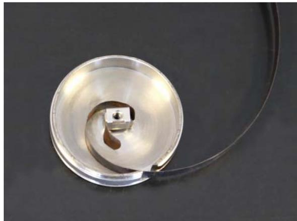
8. The end of the winding is held in place onto the center hub by a small steel clip. Pull the clip off the center hub and remove the winding. Save the small steel clip and discard the old measuring tape and winding.
