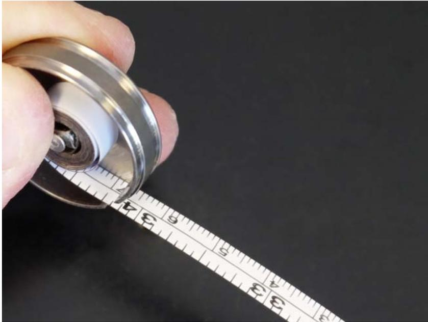
13. Once you have obtained a full 36" of measurement length, allow the tape to retract back into the housing. Carefully remove the screw from the center hub, place the cover over the housing, and reinstall the screw. Make sure to press down firmly with the wrench into the screw head while rotating clockwise, being careful not to strip out the screw socket.
