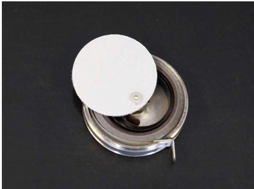
5. With the disc rotated opposite the exit groove in the housing, pull the tape up and begin to rotate it out of the housing in a clockwise manner. Rotate the guard disc at the same time so that it is opposite the tape exiting the housing. If you feel the disc difficult to
