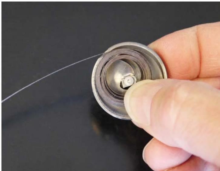
12. At this point, we can check the measurement length and tension of the tape. Hold your thumb over the housing to retain the tape during the measurement check. Pull the end tab of the tape **straight out** from the housing as far as you can to determine if you can reach 36 inches.
